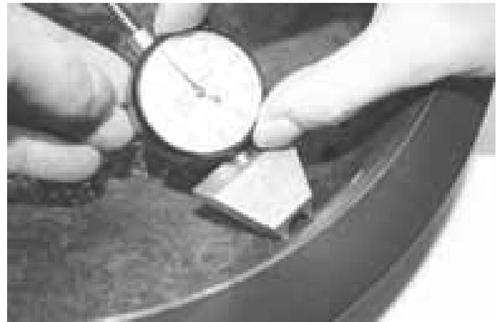
Like all Western Instruments Pit Gauges, the Pocket Pit Gauge can be equipped with an Imperial or Metric Dial Indicator or with the Digital Indicator upgrade. The accuracy and resolution for each model can be found on our Dial Indicator Specification document.
