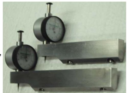
Another benefit of the cut-away on all of the Reaching Models, is the ability for the Gauge to reach over the Weld reinforcement (cap) from one side of the weld. This reach serves two purposes; first to measure weld misalignment, and the second to measure undercut on both sides of the weld without repositioning the gauge.
