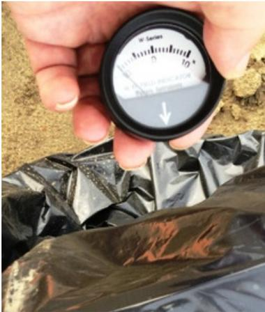
The picture to the left shows a W-FI-10 measuring a strong Magnetic Field at the end of a pipe from about 4" away from the end. We know it is strong field as we know magnetic fields drop logarithmically as a function of distance.
