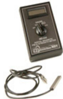
The area a Hall Effect measures is very small, while a Pocket Magnetometer is much larger. When it comes to Demagnetization we want the larger picture, as it's affect on MWD Instrumentation, and prior to Welding is far more appropriate.
