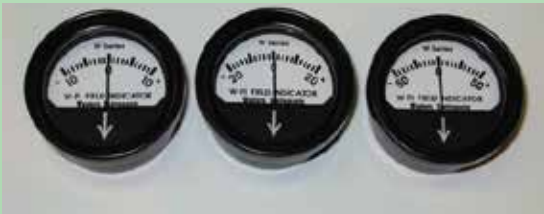
W-FI, Pocket Magnetometers W-FI-10, W-FI-20, W-FI-50 available with certification
