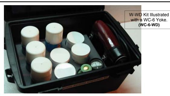
Western's MPI Kits are offered in a great variety of configurations. Our Wet / Dry Method Kit is supplied in our standard #6 Case. Our part number for a WC-6 Wet / Dry Method Kit (as illustrated above) is WC-6-WD. However, any model of Yoke can be supplied and upgraded with a W-WD to our standard #6 Case, which provides ample room for:
