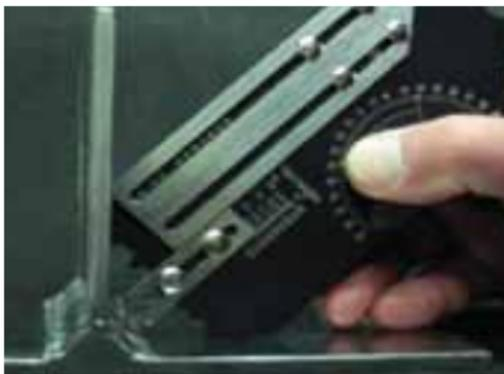
The Tri-Weld® Gauge has a large Weld Clearance Cut-away, which enables it to reach across a Weld to measure misalignment, or up to a reinforcing pad to measure its thickness.
