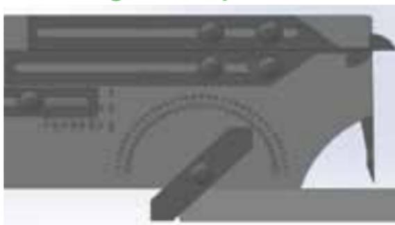
Angle of Preparation is measured using the protractor pointer, and can be used on either side of the Pointers Pivot. The Protractor is divided into  $2.5^\circ$  increments, with a common compound angle of  $75^\circ$  ( $37.5^\circ \times 2$ ) indicated.
