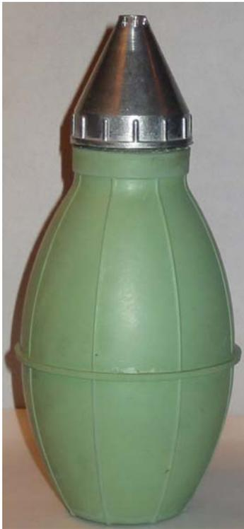
The W-PB-12 was originally a liquid glue applicator, with its Brass Tube Spigot and Rubber Cap, as shown in the picture below. At least 40 years ago, some oilfield inspector saw that it's original parts could be modified to become a Powder Bulb. The spigot is removed and its hole blocked with a special fastener.
