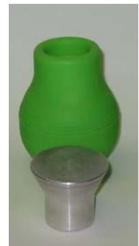
The W-PB-4 Bulb is manufactured from Silicon Rubber, so it's characteristics will not change with temperature extremes. Often, at extremely high ambient temperatures competitive Powder Bulbs become soft, limiting the dispersion of iron powder. In extremely low temperatures, competitive Powder Bulbs get hard and are easily cracked.
