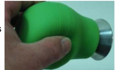
The picture to the right is the Powder Bulb in Operation. The inspector holds the Powder Bulb in a comfortable manner, between the thumb and opposing fingers, as illustrated. The cap and Screen, on the aluminium cap, are pointed toward the workpiece and the bulb is squeezed rapidly in short abrupt hand movements.
