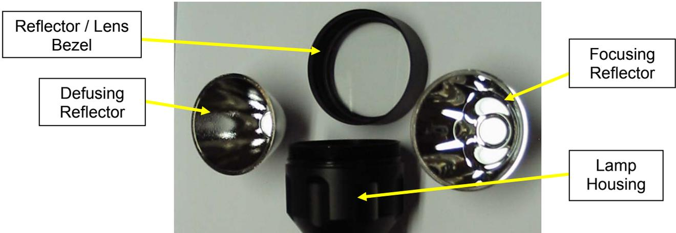
prevent the lens from dropping. The existing Reflector is then simply remove the other Reflector is installed. Operators should try both reflectors for particular inspections that may differ from background light, part geometry, etc.
