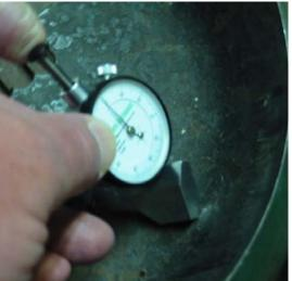
measure the pit on the complex curvature, like our vessel head above. If the shape of the surface changes from the original zero, then the Pocket Pit Gauge should be re-zeroed.
