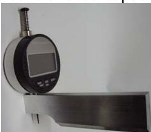
If the workpiece is configured with a Riser, Gusset, or Reinforcing Pad, the inspector simply rotates the Dial Indicator by 90°, re-zeros, and can measure up to 9.5mm (¾") from the obstruction. This ability is illustrated to the right with a Digital Reaching Pit Gauge (N88-5-D). How much the Dial Indicator is rotated, does not affect the operation of the Pit Gauge.
