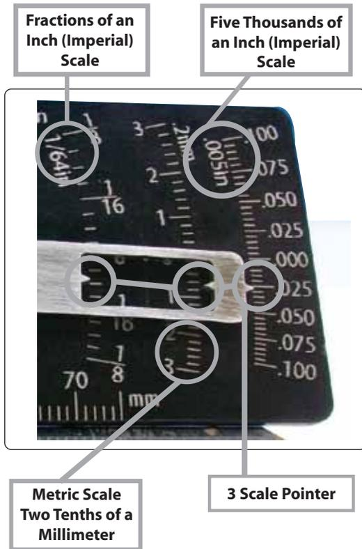
To gain resolution divisions on all scales of the Jr. Tri-Gauge are fine. Conversely these scales are linear, so estimating half measures in practice is acceptable.
