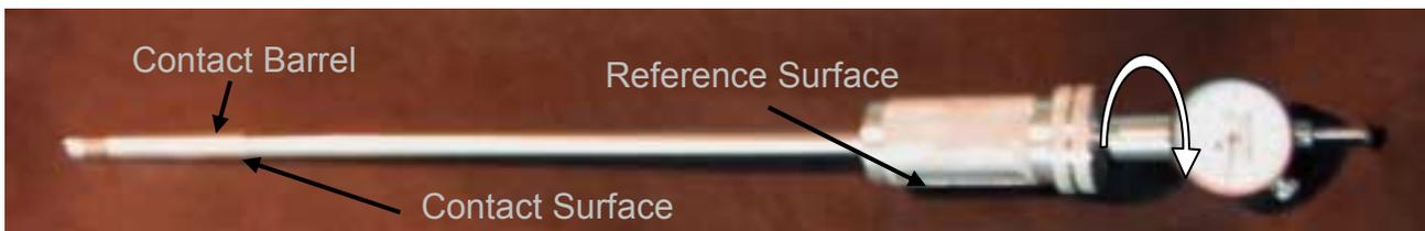
The Contact surface, from where the Contact Point extends, is simply aligned by the operator, against the target point. A reference surface (flat) is positioned on the Dial Indicator Mount, to provide the operator with a visual and physical reference for his radial position.
