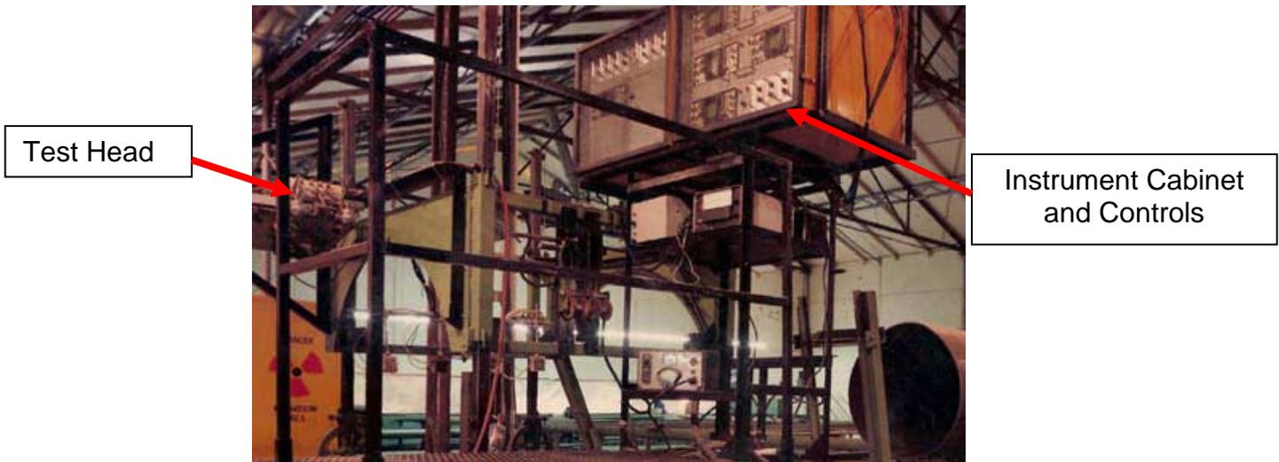
**5 Channel Straight Seam DSAW Testing System.**
