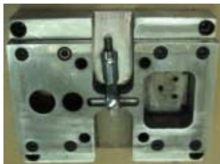
The top surface of the Shoe, mates with the bottom surface of the Probe. The Shoe has cavities and passages for Couplant and Coolant. The Shoe is also equipped with a receptacle for the Rod End's Single Point Suspension Mounting Shaft, as well as major clearances for the Rod End itself. With the downward pressure applied to the Probe/Shoe Assembly by the Oscillator Assembly's Angular Lift-off Cylinder, the Shoe follows the contour of the OD
