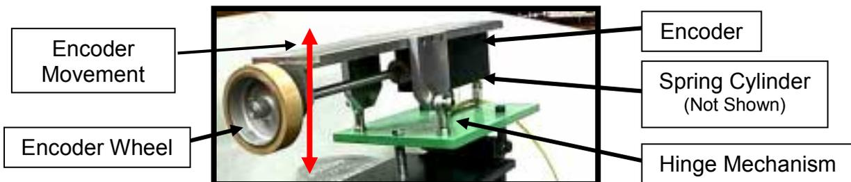
The Encoder and the mounting mechanism should be cleaned on a regular basis, simply because they are Electronic Components, and to ensure the Encoder wheel is allowed to move freely. The Encoders, at rest, should never be much more than 13mm (0.500") above the Pass Line of the Mill/Conveyer, as the
