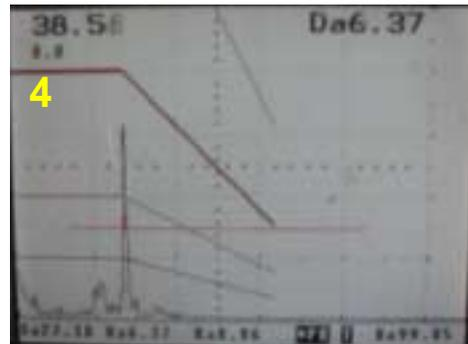
The A-Scan marked 3 shows a low level indication produced from the left side of the indication in picture 1. While A-Scan 4, shows a higher level indication produced from the right side of picture 1. If the extra 6dB of gain were removed, the indication in picture 3 would be 50% lower, and the same holds true for A-Scan 4. This reduction in sensitivity would make the indications below a Reject level.
