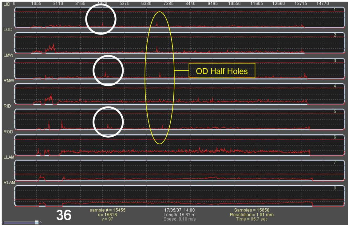
We can see that only our Left Channels show an indication, however they are all well below the reject threshold of 80% of the full screen height. The OD Half Hole has produced a higher indication on the OD channels, which is due to 2 factors; the extra reflective area of the Apex; and the compound angle (transverse and longitudinal) was not as great.
