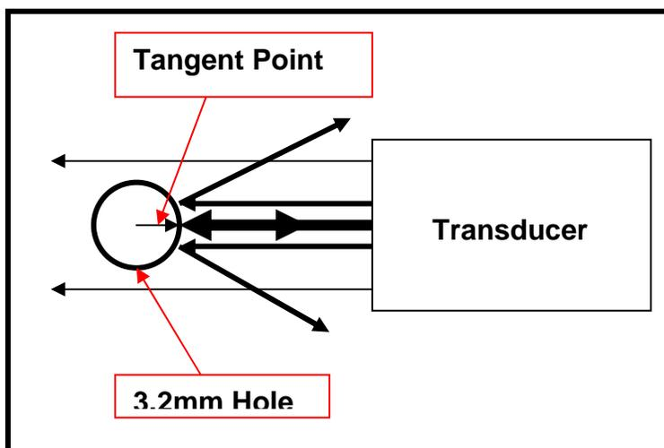
This diagram illustrates the reflective area of a hole. In our example we assume that the hole has been drilled 'Normal' to the surface. The sound that impinges on the Tangent Point of the hole, is reflected back to the transducer. The sound that impinges away from the tangent point, reflects away from the transducer. Calculations have shown that a 3.2mm diameter hole has an effective tangent area of 0.5mm in width. Thus the area of a through hole is 0.5mm times the wall thickness
