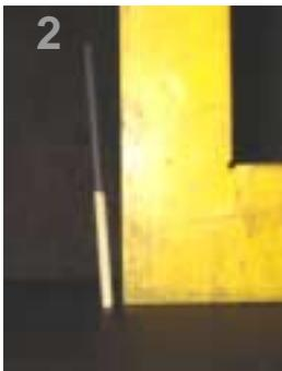
To illustrate the longitudinal angle (2), it is very easy to place a square within the picture. This angle, like a perpendicular hole, would illustrate a Penetrator or other type of Weld Interface defect. Again however, such a hole would be difficult to reproduce and would have little benefit. The 'trick' for drilling a hole, is to make it normal to the surface of the pipe.
