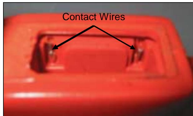
Note: If one (or both) of the contact wires is missing and the area around the wire is burnt, it is a telltale sign that the Yoke has been connected to 110 Volts DC. This power is found on old engine driven Portable Welders and some Merchant Ships.
