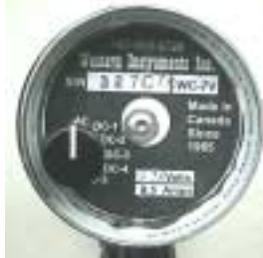
The picture to the right shows the controls of a W-7 and the WC-7, with the AC/DC field selection switch. To the left is the variable model with the AC position, and 5 preset levels of DC.
