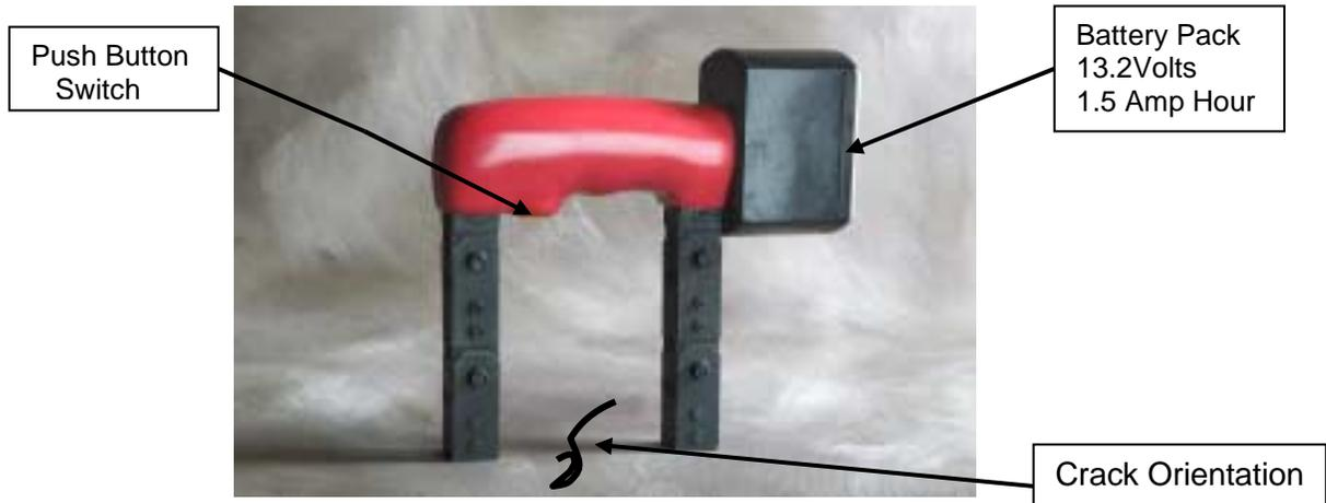
**1. Push Button Switch** – The Push Button Switch was designed for comfort and safety. While depressed, the switch delivers power (13.2 Volts DC) to the coil encapsulated in the Yoke housing.
