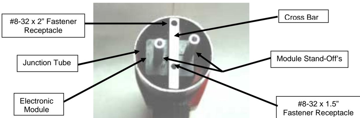
The Module is fitted with 2 Aluminum Stand-Off's that permit the connection of the Battery Assembly to the Module. The Cross Bar is used to secure the Battery Pack Assembly, and has 2 holes, one drilled through (top), and the lower one threaded for an 8-32 fastener.
