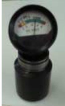
**Battery Meter measuring Battery under load.**
