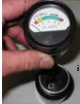
**Inserting Meter into Battery Plug**
