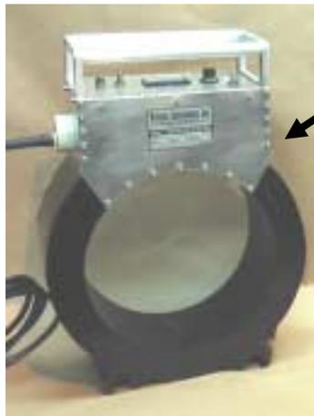
DC End Area Demag Coil
