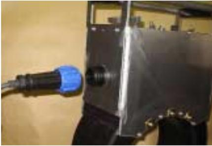
One of the most common repairs to Portable Equipment is the Power Cord becoming damaged by accident or careless operators. In an attempt to mitigate these mishaps, WD-Series Coils are offered with Removable Power Cords. As illustrated to the left, a male connector is installed into the Controls Housing, and accepts the female threaded Connector.
