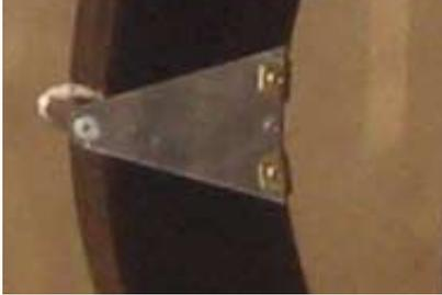
ID Wear Bars are Clamped to the Coil, so they can be positioned at any point around the Coil.
