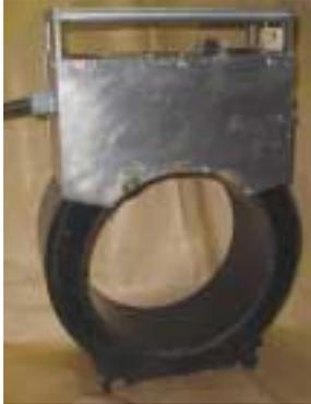
The WDV-10 shown here, has been in field service for 2 years, and was equipped with ID Wear Bars prior to being delivered to the customer. ID Wear Bars are made of Brass, so they won't damage the part under test, and will slide easily on the workpiece.
