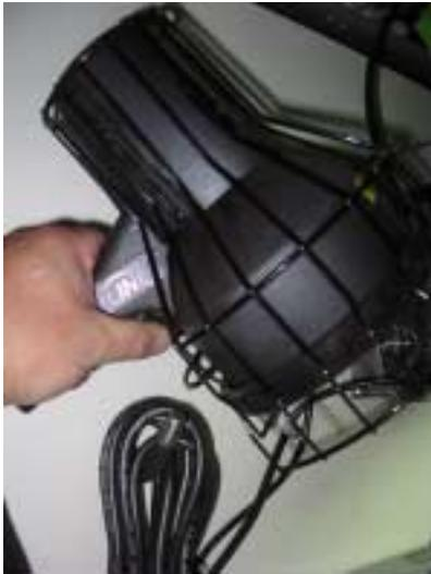
The view of the UV Lamp to the left, shows the Booth's receptacle for the Lamp, with the excess power cable neatly wrapped and hanging on it. The view to the right shows the lamp sitting face down on the work surface. It is recommended to keep the UV Lamp on the receptacle at all times. It is acceptable to set the lamp face down for short periods of time during an inspection. If the bath is allowed to splash up onto the
