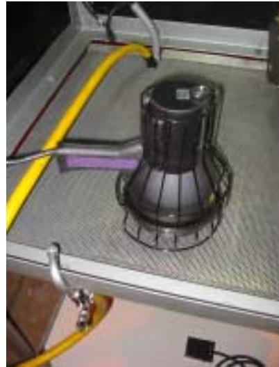
Lamp's Lens, it will either break or explode outwards, causing great risk of burns to the operator and affecting the cleanliness of the bath.
