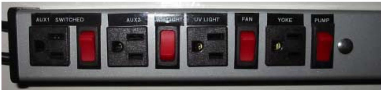
1. Pump Switch. Turns on and off the supply / agitation pump.
