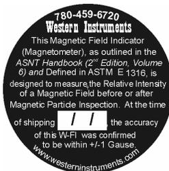
"This Magnetic Field Indicator (Magnetometer), as outlined in the *ASNT Handbook (2<sup>nd</sup> Edition, Volume 6)* and Defined in ASTM E 1316, is designed to measure the Relative Intensity of a Magnetic Field (measured in *Gauss*) before or after Magnetic Particle Inspection. At the time of shipping \_\_\_/\_\_\_/\_\_\_, the accuracy of this W-FI was confirmed to be within +/-1 Gauss or 5% of the scale value, whichever is greater."
