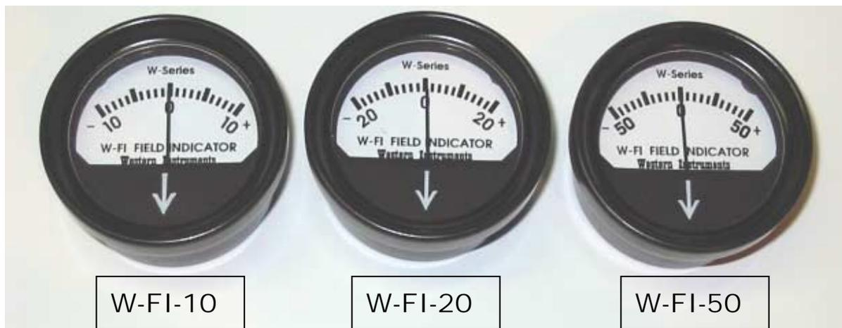
A magnetic field of under 10 Gauss is typically not strong enough for Magnetic Particle Inspection (MPI), thus the W-FI-10 is used to ensure a workpiece is demagnetized after testing and before further processing. A magnetic field, for MPI, should be
