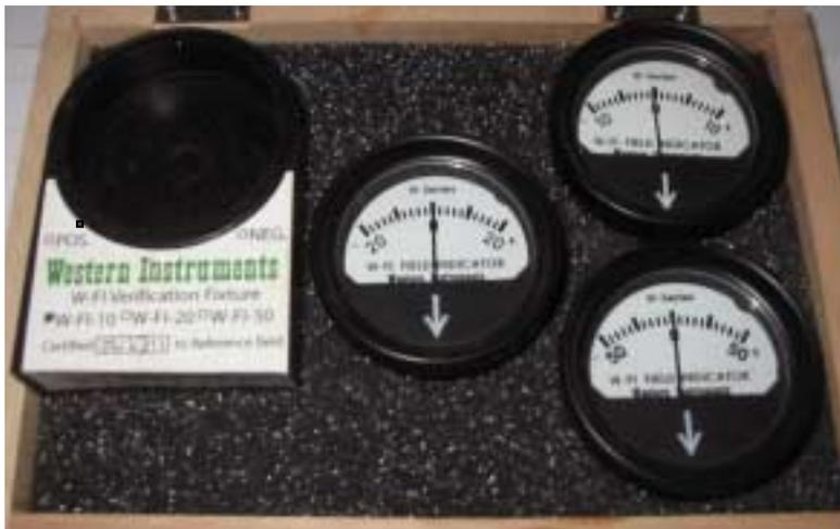
When any of the W-FI's are placed into the W-10 Verification Fixture, they will indicate a 10 Gauss field. The picture below, shows a W-FI-20 in the W-10, indicating a 10 Gauss Field. Another feature of our Verification Fixtures, is we offer them in either Positive or Negative ranges. Some Customers, with large
