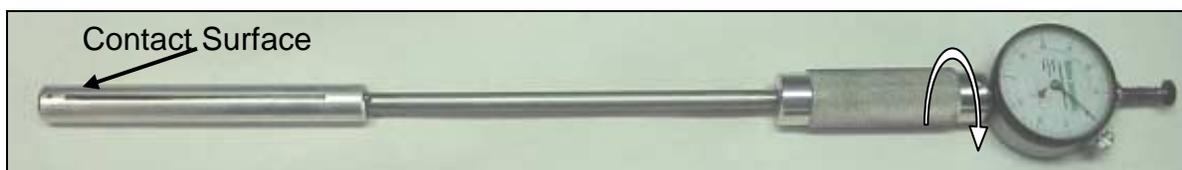
The Contact Surface, from where the Contact Point extends from the Barrel, is held up against the target point by a leaf spring, extending for the opposite side of the Barrel. The Hold Down Spring is changed to compensate for larger sizes of tube, with the practical limit being 3" (76mm). The *Tube Sheet Pit Gauge*® has a measurement range of 0.150" (3.8mm).
