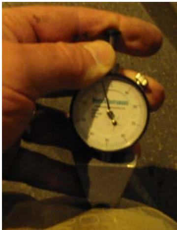
With the Dial indicator installed on The Pocket Blade, it is used for Inspecting areas with complex curvatures, such as the base or neck of the cylinder. The picture to the left, shows the Pocket Pit Gauge measuring the depth of the stamped identification lettering on the neck of a Nitrogen Cylinder. As the name suggests, the Pocket Pit Gauge conveniently fits in your pocket, unlike the Reaching Plus Pit Gauge.
