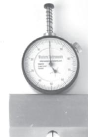
For more accurate Pit Depth Measurement, Western Instruments offers Dial Indicator Pit Gauges (Imperial, Metric, & Digital). These Pit Gauges are also designed for more specific applications, such as Weight Loss Corrosion, Corrosion Coupons, and more complex geometry's.
