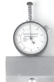
For more accurate Pit Depth Measurement, Western Instruments offers Dial Indicator Pit Gauges (Imperial, Metric, & Digital). These Pit Gauges are also designed for more specific applications, such as Weight Loss Corrosion, Corrosion Coupons, and more complex geometries.
