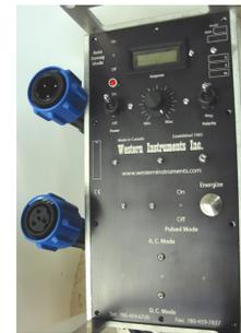
The only visible difference between a Remote Control Panel and a standard Coil Mounted Panel is the Switch Boots. Due to the higher Amperage requirements of a large diameter Coil, the switches need to be larger, which requires different boots. However, inside the Remote Control Housing, and mounted to the underside of the Control Panel, are the larger capacity
