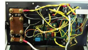
Remote Control Power Supplies are fitted with a safety interlock, where the Polarity Switch is mechanically held for 2 seconds after the energize button is released. If a careless operator attempts to excessively force the Polarity Switch in that 2 second envelop, he will break the switch housing, at a minimum. If he succeeds in latching the switch in this manner, there will be a great deal of damage to the Control Panel.
