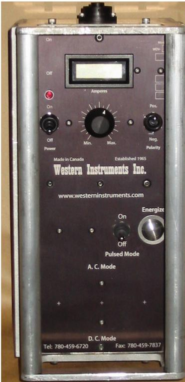
One of the many benefits to WD-Series Coils are the Self Contained Controls, however for larger Coils, where they are a little heavy to be handled by a single operator, Western offers Remote Controls. The curved lower portion of the Control Housing is removed, and a solid bottom is Welded in to form the bottom of the light and rugged housing. This allows operators to move around the workpiece and having full access to the controls.
