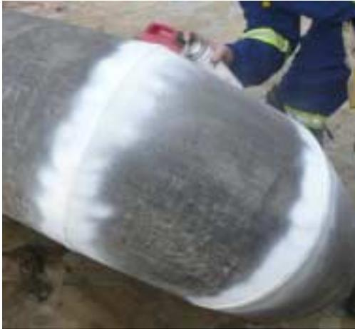
The picture to the right shows an inspector applying White Contrast Paint to a Boiler Fire Tube in the field (note surface finish). A specialized crew would use bulk application system, due to the area needed to be covered, however this application is by more expensive aerosol cans.
