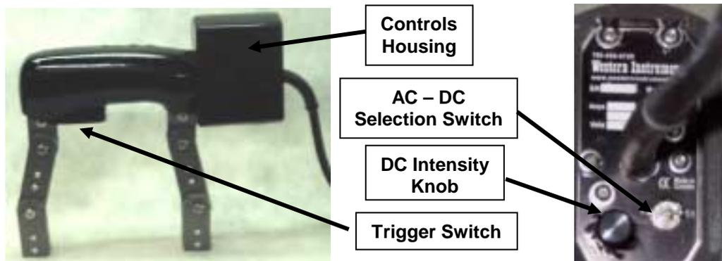
other AC Yoke. When the DC Field is selected, the line voltage is reduced (in the form of heat) and rectified to produce a DC wave, often referred to as Half Wave DC, or Pulsed DC. This form of DC provides the best Particle Mobility of any type of DC magnetization, but it is still not as good as AC. Here again DC will find slightly subsurface defects while AC only works on surface breaking defects, which in essence is the benefit of an AC/DC Yoke.
