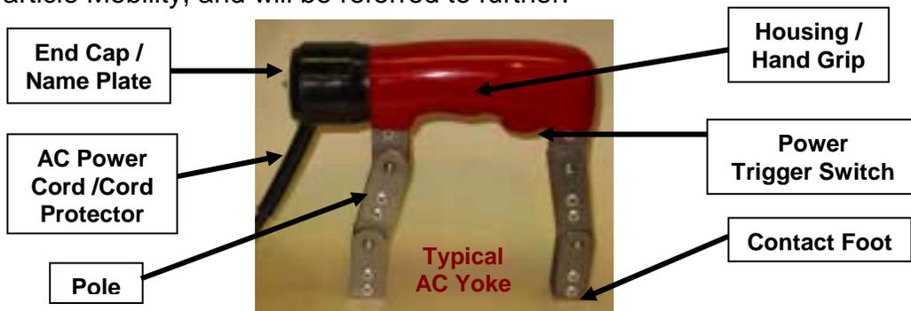
AC Yokes must lift a minimum of 10 Pounds or 4.6kg, which requires the Feet to be placed squarely on a Pull Test Bar (W-PT), thus permitting as much magnetic field as possible to flow through the bar. Thus when the Yoke is placed on a curved surface the operator must ensure that as much of the foot as possible is contacting the workpiece. A properly maintained AC Yoke, with the feet ground flat, will lift the Pull Test Bar if the feet are at their maximum or minimum distance.
