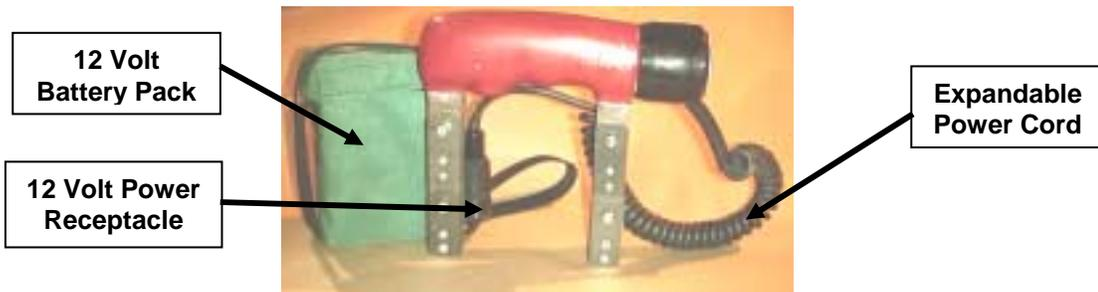
A 12 Volt Battery can be used on an AC Yoke, but it will overheat very quickly while lifting 100 pounds! When a conventional AC Yoke is connected to a 6 Volt Battery, it will not heat as fast and will still lift 50 pounds.
