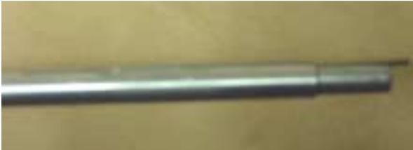
Insert the Contact point into the Slot on the Contact Surface Housing. Bring the Contact Point to the extreme Bottom End of the Contact Surface Housing, but leave a short length protruding past the end (as illustrated to the left). The Retainer Tube is then slipped over the Contact Surface Housing.
