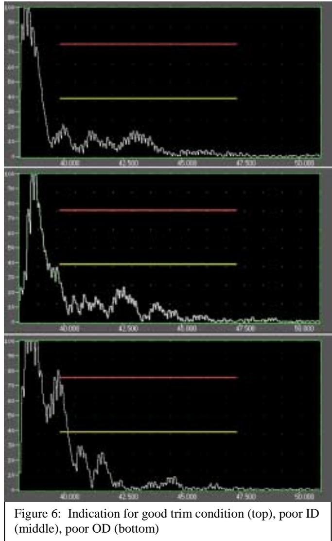
This is the best way to ensure the optimum signal quality, performance and repeatability in a mill testing environment. Where ideal trim conditions are a requirement, a Flash Gauge can be utilized. A Flash Gauge gives a continuous cross-section of the weld area. That is, the Flash Gauge draws an ID and OD profile of the weld area and gives instant feedback of trim conditions. This is highly desirable as corrective action can be taken without delay.
