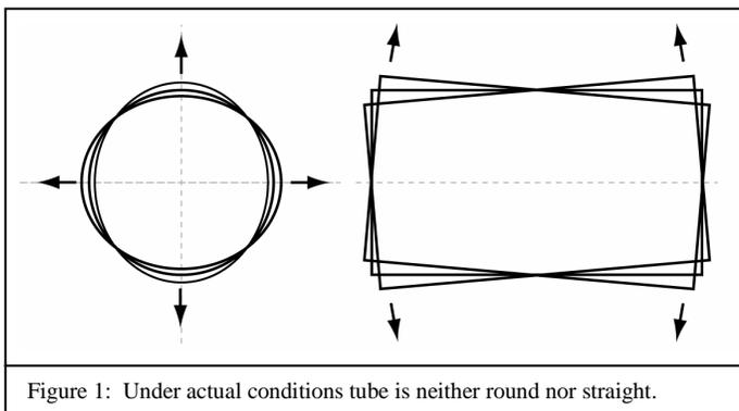
Figure 1: Under actual conditions tube is neither round nor straight.
