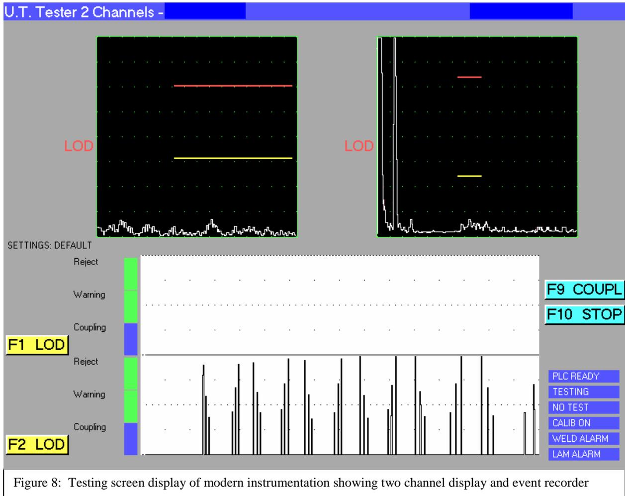
Figure 8: Testing screen display of modern instrumentation showing two channel display and event recorder
