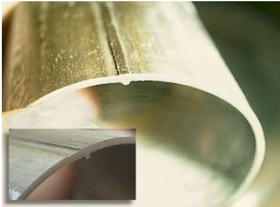
Figure 5: 1.25" Dia. x 0.028" with poor trim conditions
