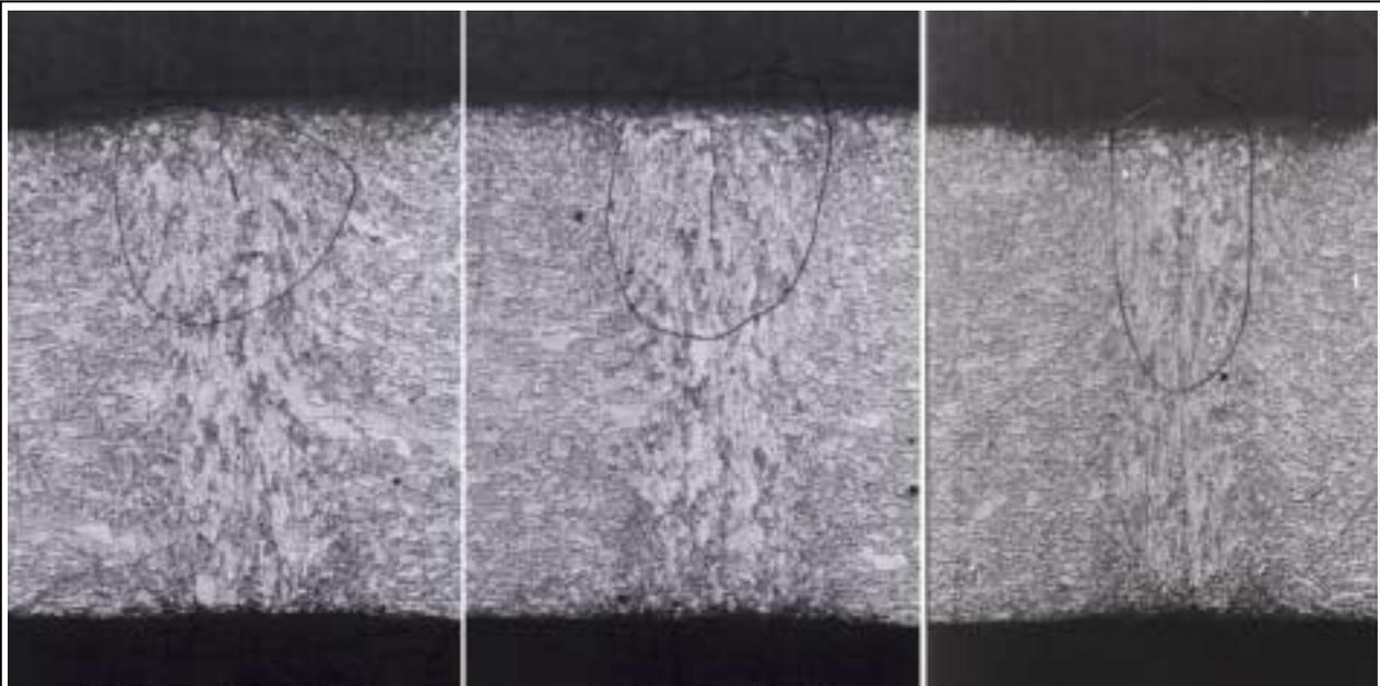
Figure 4: Defects detected on 2" Dia. x 0.054" tube are approximately 19 - 46% of wall thickness.
