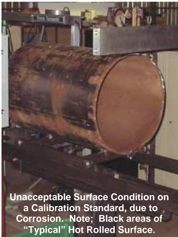
**Unacceptable Surface Condition on a Calibration Standard, due to Corrosion. Note; Black areas of "Typical" Hot Rolled Surface.**
