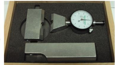
Specified by a Senior Vessel Inspector, the Pocket Pit Gauge allows inspection on complex curvatures, such as the Knuckle Area on Vessel Heads, and even pump housings and impellers. As the name suggests, the Pocket Pit Gauge conveniently fits in your pocket (but then again so does the Basic Pit Gauge).
