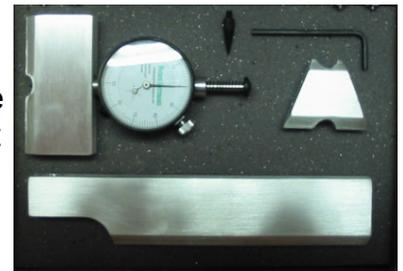
Specified by a Senior Inspector, the Pocket Pit Gauge allows inspection on complex curvatures, such as the Knuckle Area on Vessels, and other complex curvatures, such as pump housings, valve bodies, impellers, turbine blades, etc. As the name suggests, the Pocket Pit Gauge conveniently fits in your pocket (but then again so does the Basic Pit Gauge).
