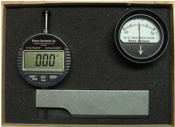
The Reaching Pit Gauge has been selected because Yellow Jacket (and other coatings typically end far enough back from the weld that the coatings don't interfere with the Reaching Blade sitting flat on the Pipe surface. The cutaway nose, on the dial indicator end of blade, permits positioning the Dial or Digital Indicator's Contact Point on either side of the weld.
